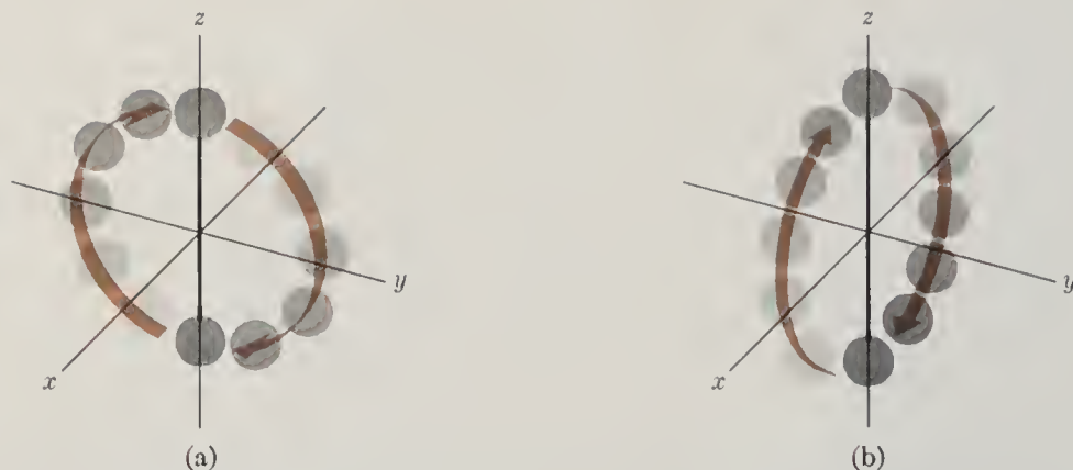
FIG. 2.15 Rotational motion of a diatomic molecule. (a) Rotation about the x-axis. (b) Rotation about the y-axis.
