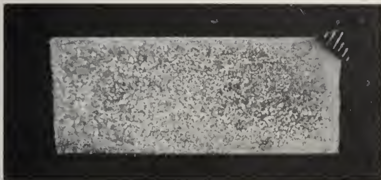
Etched surface of copper showing microcrystalline structure.
