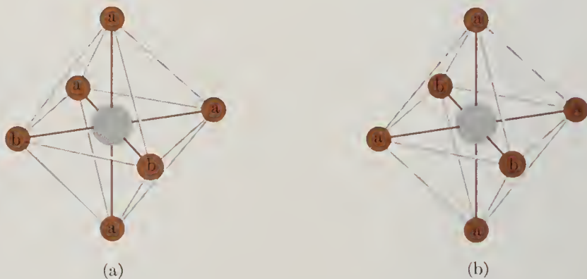
FIG. 16.5 Geometrical isomers of octahedral Ma_4b_2 complexes: (a) cis isomer, (b) trans isomer.
